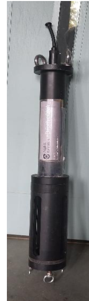
Figure 3 The inDepth sampler contains a high-volume pump (top compartment) and enables the collection of eDNA on a filter cartridge housed in the protective cage (bottom compartment).
