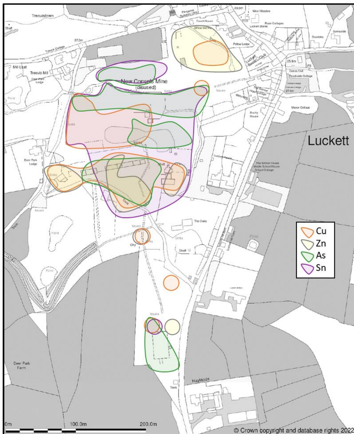
Figure 4-28 Site plan highlighting areas of Cu, Zn, As and Sn concentrations in the upper quartile of 94 surface soil and mine spoil samples obtained on NGC during May and June 2023 (full data displayed in Figure 4-16 to Figure 4-19). Map base supplied by mapserve.co.uk a licensed Ordnance Survey partner (100053143). © Crown copyright and database rights 2023 Ordnance Survey 100049047.
