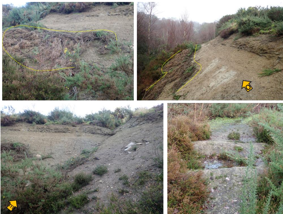
Figure 4-4 Illustration of physical processes that slow down natural revegetation of spoil heaps and tailings: surface erosion of steep slopes and compaction on paths due to recreational use (footfall, biking, bottom right). Compare also with images shown in Figure 3-2. Top row: yellow outlines show areas where cut vegetation has been placed on the slope. Yellow arrows correspond with viewing angles in Figure 4-1. Photos: C Braungardt 2022/3.
